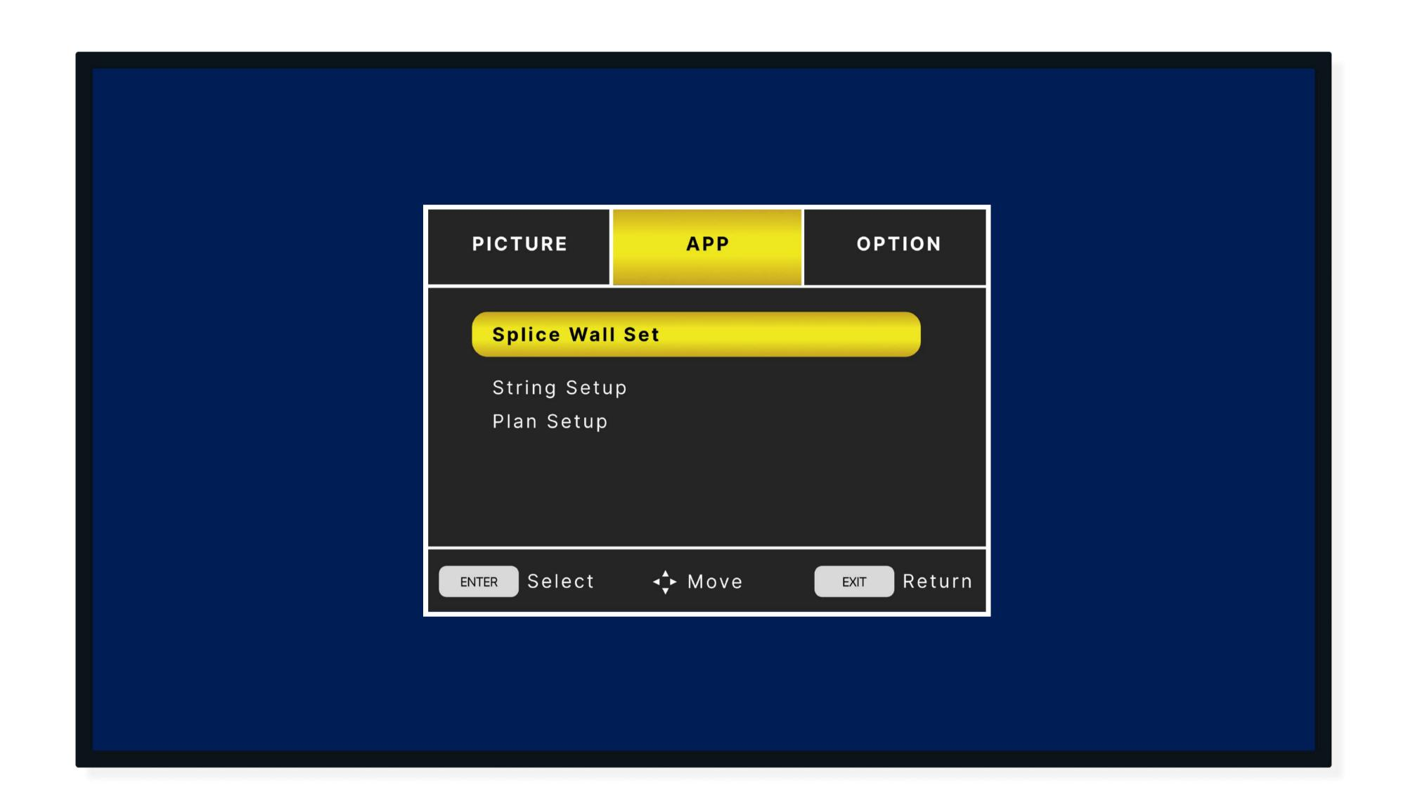
Under the "Application" menu, press "UP / DOWN" to select "Stitching Settings" in turn, press "ENTER" to enter "Stitching Settings", then press "LEFT / RIGHT" to set splicing, and then press "ENTER" to confirm ,As shown in the fiture to the right.
